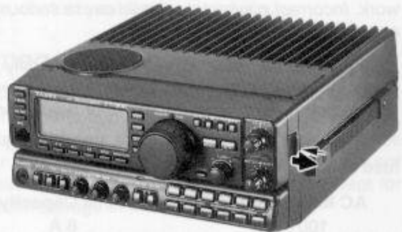
Removing the Front Sub-Panel
