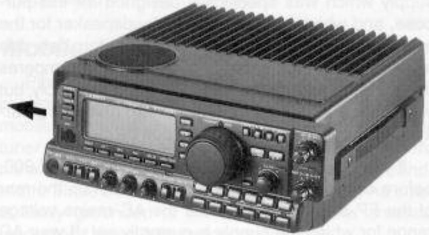
Installing the Front Sub-Panel
