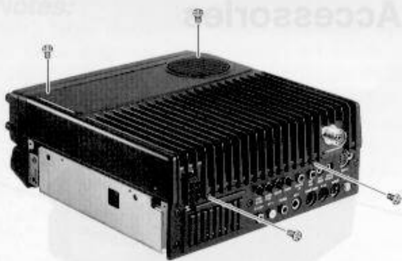
Fig. 4: Top Cover/Heatsink Removal
