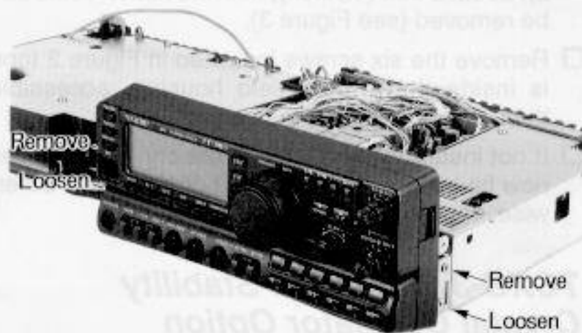
Figure 7: Front Panel Screws
